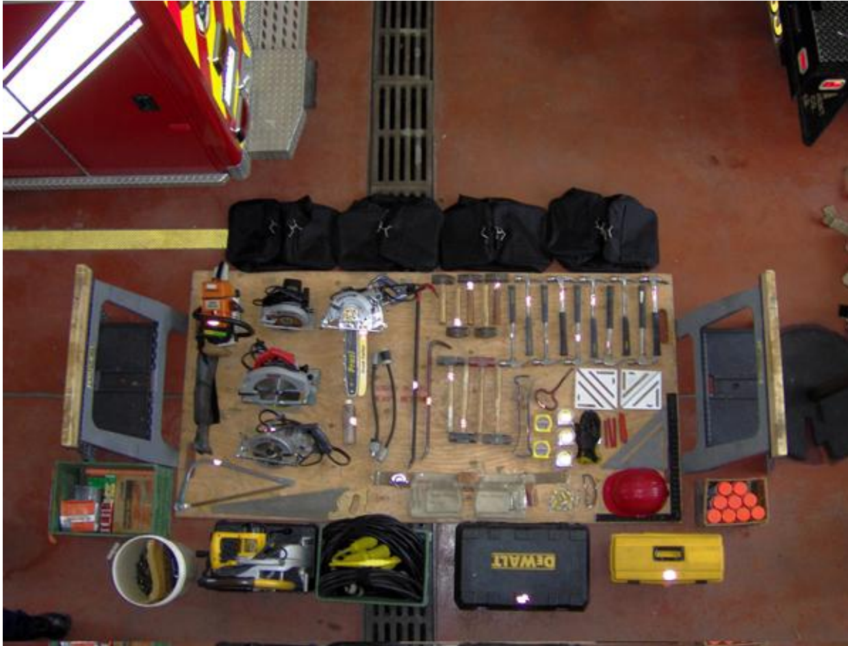
Figure 10-9 Small tools and gear used in trench rescue
